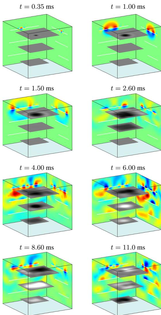
Figure 2: Acoustic pressure propagation generated by a strike on the upper plate, at times as indicated. Central cross sections of the acoustic field along the  $xz$  and  $yz$  planes are plotted, as well. The projections of the plates on these planes are marked with white lines.
