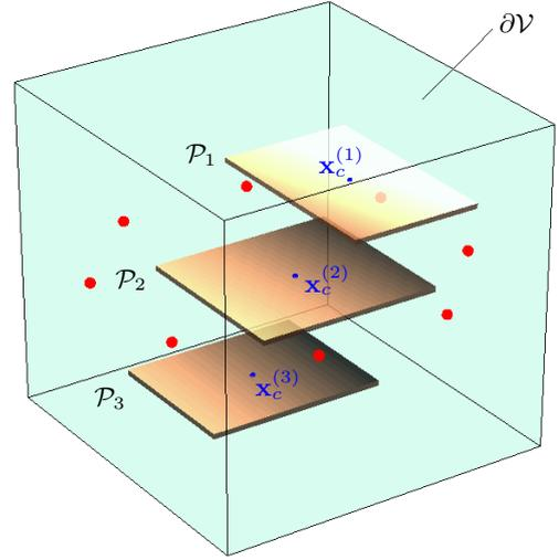
Figure 1: *Geometry of the model. Three plates  $\mathcal{P}_1$ ,  $\mathcal{P}_2$  and  $\mathcal{P}_3$  are embedded within a 3D box  $\mathcal{V}$ . The boundary of the box is indicated with  $\partial\mathcal{V}$ . Centre positions for every plate are marked with their coordinates  $\mathbf{x}_c^{(i)}$  (in blue). Possible output locations are marked with a ring of bold dots (in red).*
